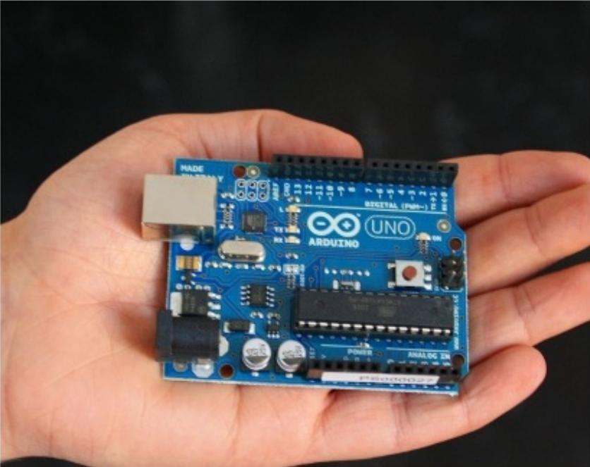
Arduino is an open-source electronics prototyping platform based on flexible, easy-to-use hardware and software. It's intended for artists, designers, hobbyists, and anyone interested in creating interactive objects or environments.
